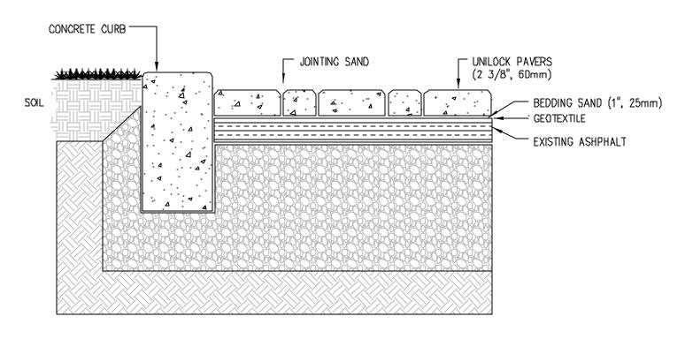
NOTE: It is possible to lay pavers over existing ashphalt if the base is in good condition. Adjacent soil or lawn may have to be built up.
